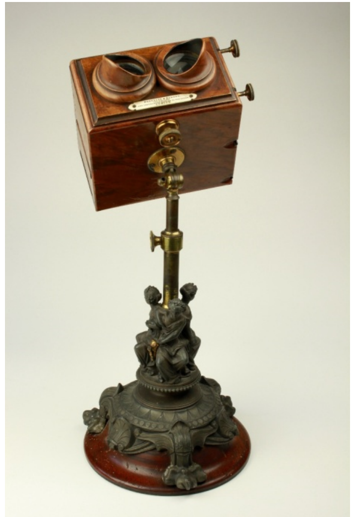
1148 Victorian walnut cased Negretti & Zambra stereoscope, on an adjustable pole raised on a three legged cast metal stand depicting three females, further mounted on a mahogany base, original makers label to front of stereoscope, reads 'Negretti & Zambra, Opticians and Instrument Makers to the Queen, London', total height 53cm approx. (not extended)
