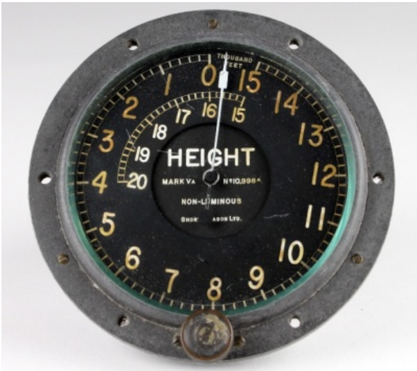
1136 Short & Mason Mark V A non-luminous aeroplane altimeter, no. 10998A, total diameter 11.5cm approx.
