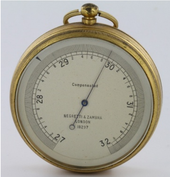
1134 Negretti & Zambra compensated brass barometer, diameter approx 6.55cm
