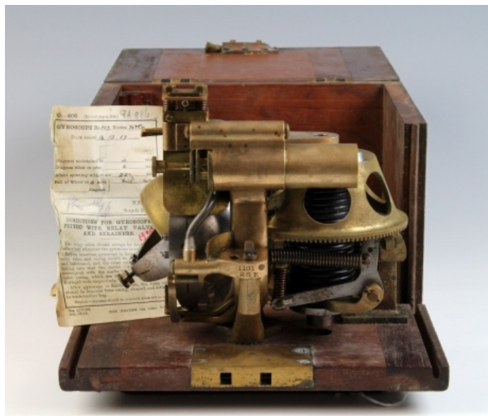
845 Gyroscope. An early 20th century brass and steel torpedo gyroscope, by 'W&Co.', stamped '1101 R.G.F.', comes with a test certificate dated 1917, contained in original mahogany case (stamped 'SD'), gyroscope height 17cm approx.
